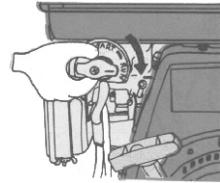
9. Push the choke to "OPEN" position as engine warms.
